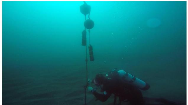
Figure 3.4. CINMS diver Ryan Freedman services a telemetry mooring anchored in soft sediment at Santa Barbara Island. Photo: Pike Spector/NOAA
